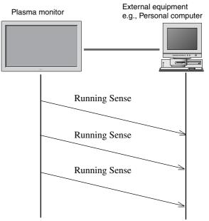
The plasma monitor regularly transmits a Running Sense command at an interval of approximately 1 second. (Running Sense command: 1FH 60H E0H 88H 00H E7H) This command is used to recognize optional equipment. The return of an ACK is not required when external equipment such as a personal computer has been connected. Note that destruction of this data is recommended when it is taken in.
